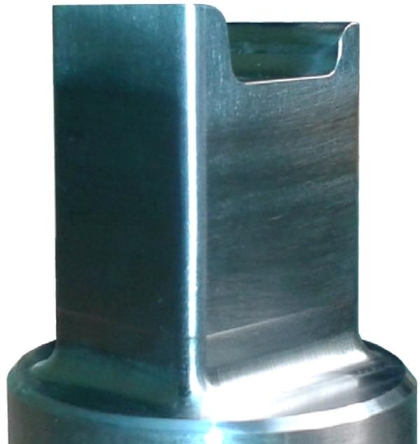
Photograph above shows component with correct finished geometry. Carbide tool held in Nikken Slim Chuck. This component would not require flattening, blending or polishing
