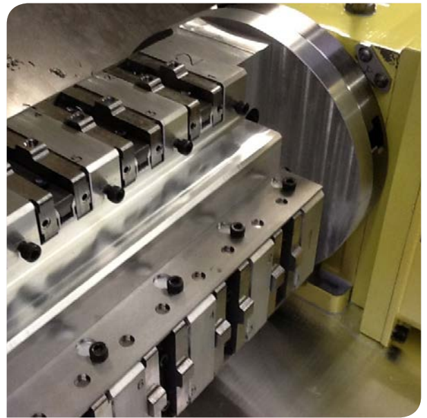
CNC202 Rotary Table with TAT170N and Trunnion Fixture Set Up.
