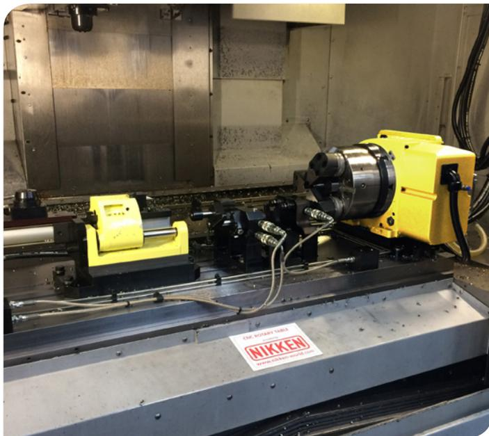
NIKKEN CNC260 Rotary Table + H170-S Hydraulic Tailstock with Hydraulically actuated workholding
